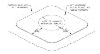
**Step 2:** Cut a patch of ALT Fleece reinforcement (circular or rectangular with rounded corners) a minimum of 4-inches (10 cm) larger in all directions of the repair area and fray all edges. A minimum of 4-inch (10 cm) overlap onto sound in-place membrane is required.
